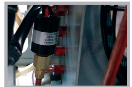
oversized condenser for high ambient temperatures oversized condenser uses a high pressure fan switch to protect refrigeration circuit
